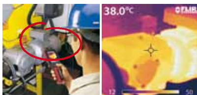
Mechanical check-up of an electrical motor using the FLIR i60.
