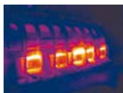
Refractory insulation defect
