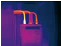
Poor connection and internal damage
