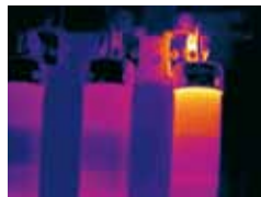
Internal fuse damage
